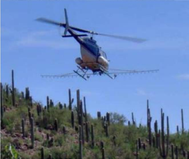
Helicopter with spray boom (USFS) Aerial application with spray ball (USFS during demo)
