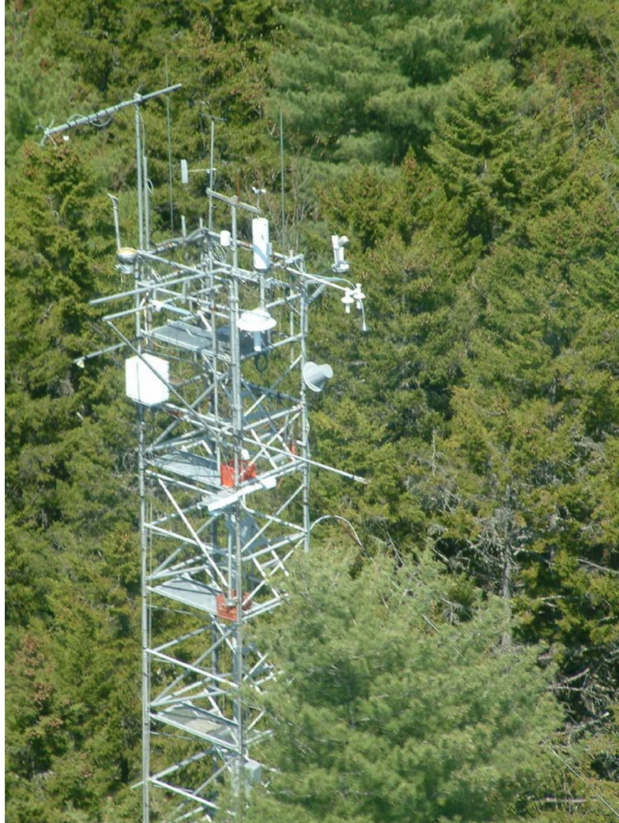
Figure 2. Mitigation of climate change impacts: Monitoring forest carbon exchange with eddy-flux towers, here at Forest Service Northern Research Station facilities in Howland Maine. The towers support the apparatus used to measure the hourly uptake and release of CO 2 by trees and the soil, to determine impacts on carbon storage by management treatments over daily, seasonal and annual growth cycles. Photo from John Lee, University of Maine.
