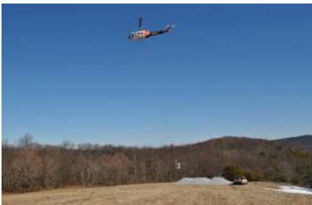
Figure 8: 3/4/13 A helicopter picks up a one ton bucket of limestone sand to deposit in Saint Mary's River. Photo credit, USDA Forest Service.
