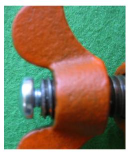
Flicker Forge 1/2"-dia. handle bolts are too short to use Roll Pins. Drill and tap for ¼-20 thread. Drill about 1/2" deep, tap, and insert a 3/8" long ¼-20 screw with a large diameter head. Hex head screws can be used.
