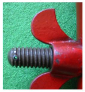
If your handle bolt is long enough, drill a 3/32" hole and insert a 3/32"-dia. Roll Pin (aka Split Pin, Tension Pin). 7/16" long roll pins are available from McMaster #98296A837 (500/box \$8.74) or use 1/2" pins and file down the excess.
