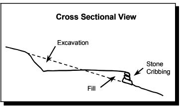
**Figure 7.** Cross sectional view of a side-hill constructed tent pad. Surface should be slightly crowned in all directions for water drainage.
